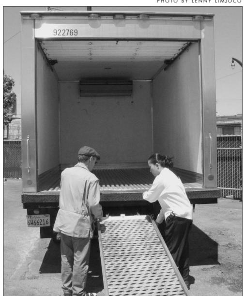
This freezer truck, which will be loaded with bags of infested items, kills bedbugs at 20 below zero for 24 hours.
